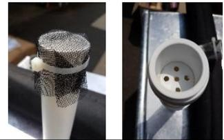
A leaf guard can be mesh attached with a cable tie or a socket plug with holes drilled in it
